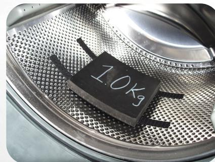
Figure 6. 1.0 kg mass imbalance placed in tub
