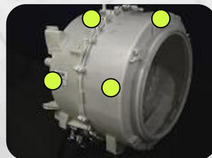
Figure 7. Accelerometer locations on washing machine tub
