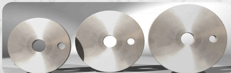
Figure 5. Aluminum ISO-8662-4 angle grinder test disks
