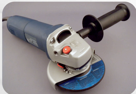
Figure 4. Sample angle grinder used for testing
